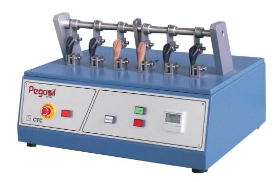
"BALLY" flexing machine with 6 stations
